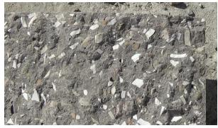
aggregates in production of self- compacting concrete. Concrete is evaluated by using different destructive and nondestructive techniques. Natural aggregates were replaced up to 50% with ceramic aggregates. Results are encouraging as compressive strength of modified concrete was more as compare to ordinary concrete. Furthermore, ceramic waste aggregates increase the compact ability as unit weight of modified concrete was more as compare to ordinary concrete.
